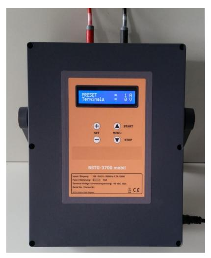
Mobile Battery String Test Generator for battery installation and service
