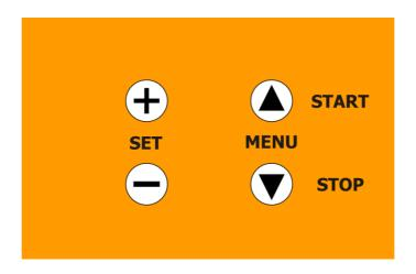
Use and to select the pre-setting (PRESET) of the desired output current from 1 A to 21 A. The figure is the sine RMS value
